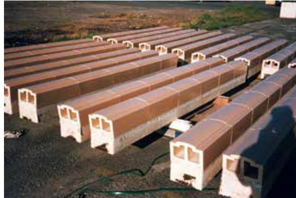
Figure 4c Terra cotta mullions.
