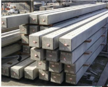
Square Piles (most common shape) Typical Shapes: 12", 14", 16", 18", 20" and 24"
